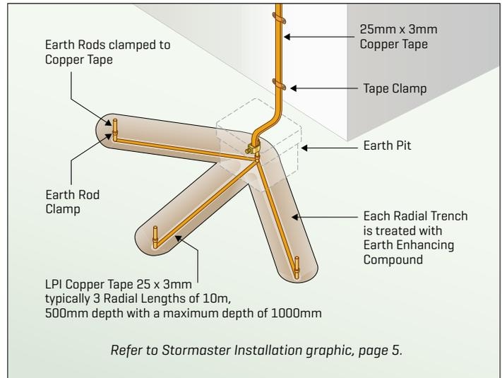
Key components of a lightning earth include:
